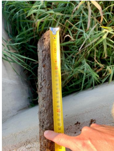
Figure 18: Sludge height in RBs Kastelir.
