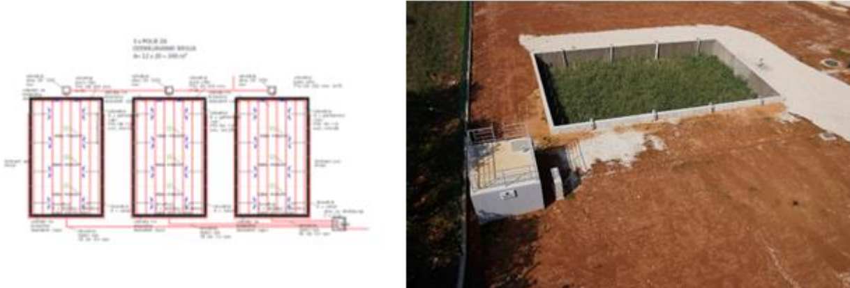
Figure 17 Floorplan of designed RBs in Kastelir (left) and the already established RB at Kastelir (right)
