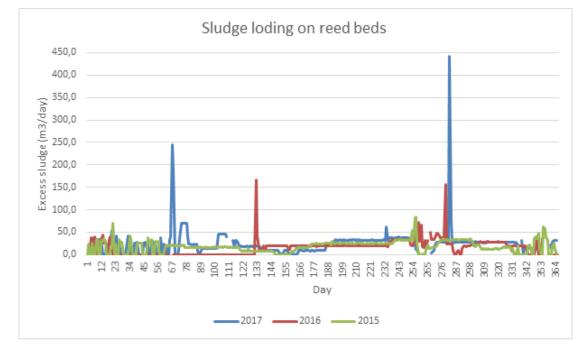
Figure 32: Daily sludge loading on reed beds in Dellach
