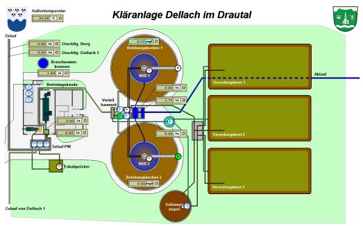
Figure 25: WWTP Dellach process scheme<sup>27</sup>
