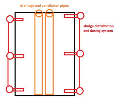
Figure 26: Sludge dosing system (red) and leachate collection system (orange)
