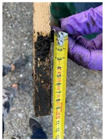
Figure 19: Sludge height in RBs Mojkovac.
