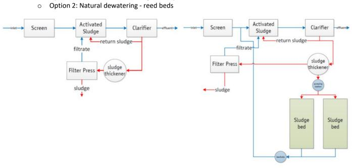
Figure 7: The process flowchart of WWTP Mojkovac with mechanical dewatering (left) and natural dewatering (right)<sup>17\*</sup>
