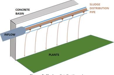
Figure 8: Sludge distribution pipe
