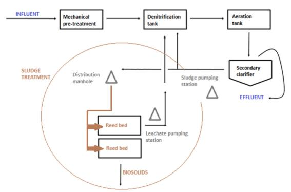
Figure 9: Flowchart diagram of operating sludge treatment in Mojkovac
