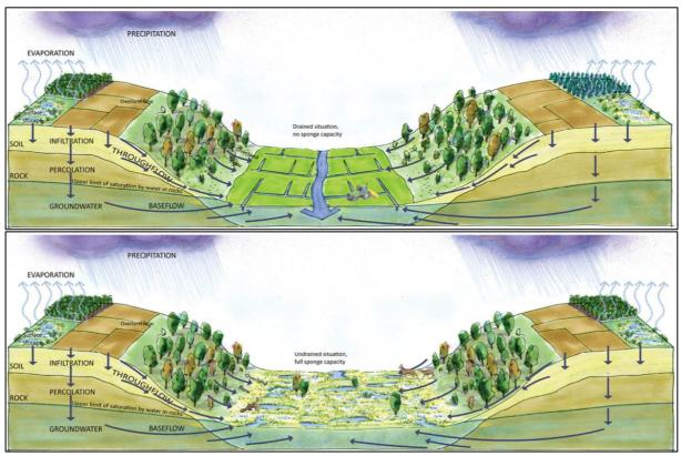
*Fig. 2.2. Systemic impression of restoration of natural water retention, before (above) and after restoration. It requires removal of existing drains, resulting in drastic reduction of discharge peaks in the upper parts of a river basin. These effects are noticeable at local, regional and (inter)national level.*
