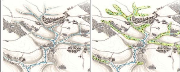
*Fig. 3.3. Restoration of natural retention in a micro-catchment. Approximately 6% of a micro-catchment is suitable for natural retention.*
