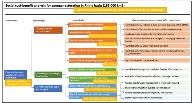
Fig. 5.1. The diagram shows, in qualitative terms, the social benefits and costs for restoration of natural water retention ("natural sponge capacity") in the Middle Mountains in Germany. Where possible figures have been added for the effects generated by the study area. These figures do not represent the full potential of natural water retention but show effects when 38% of the restoration potential is used.
