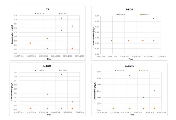
Figure 50. Graphic representation of the concentrations of the main pollutants monitored in the station PP1-A2-8 (influent) and PP1-A2-5 (effluent)
