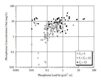
Figure 21. Outlet TP concentration versus TP loading for HF from Kadlec and Wallace (2009); data from 193 HF wetlands
