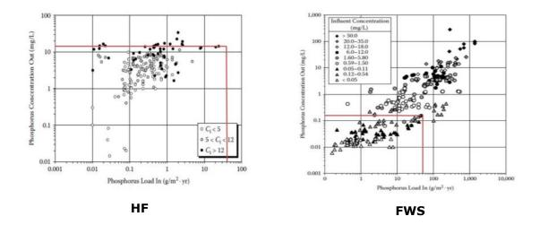
**Figure 30.** Outlet TP concentration versus TP loading for HFs (left) and FWSs (right) from Kadlec and Wallace (2009) compared with the loading rate phosphorous of the PP2 wetland basins of Marina di Latina (red lines).
