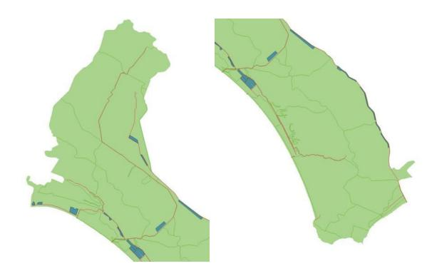
**Figure 40.** Rio Martino catchment: suitable areas for the implementation of wetlands according to suitability criterion 2 (in blue) on available areas in proximity of the main drainage canals (in red)
