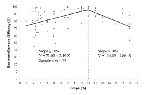
Figure 22. Correlation between sediment removal efficacy and buffer slope (Zhang et al., 2010)
