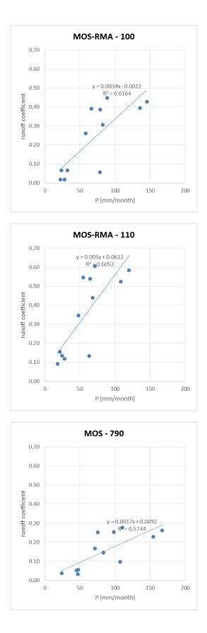
Figure 49. Linear fitting of the runoff coefficient equation for the sub-basins of interest
