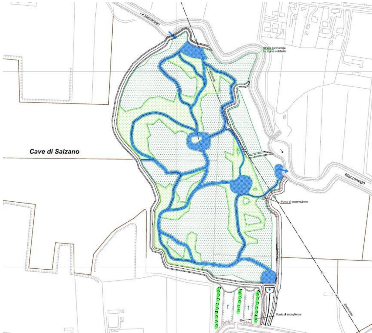
**Figure 7.** Planimetry of the Salzano wetland, built within the Salzano quarry: wood area (dark green dots); vegetated FWS area (light green dots); open water FWS area in blue.
