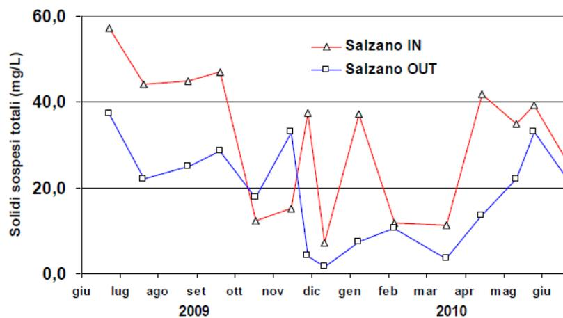
**Figure 46.** Influent and effluent TSS concentration for the Salzano wetland.
