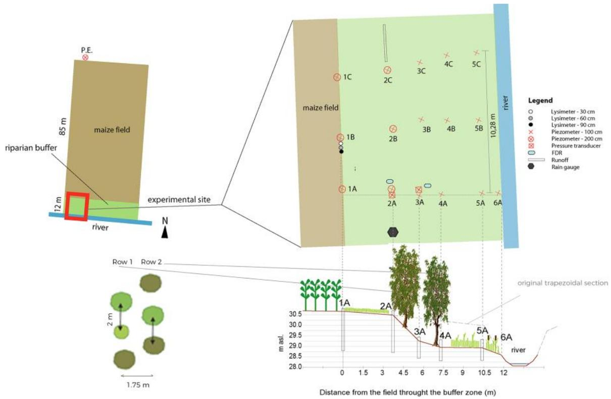
**Figure 10.** Illustrative design of the Scandolara buffer strip, including indications on the experimental scheme (modified by Gumiero & Boz, 2017)
