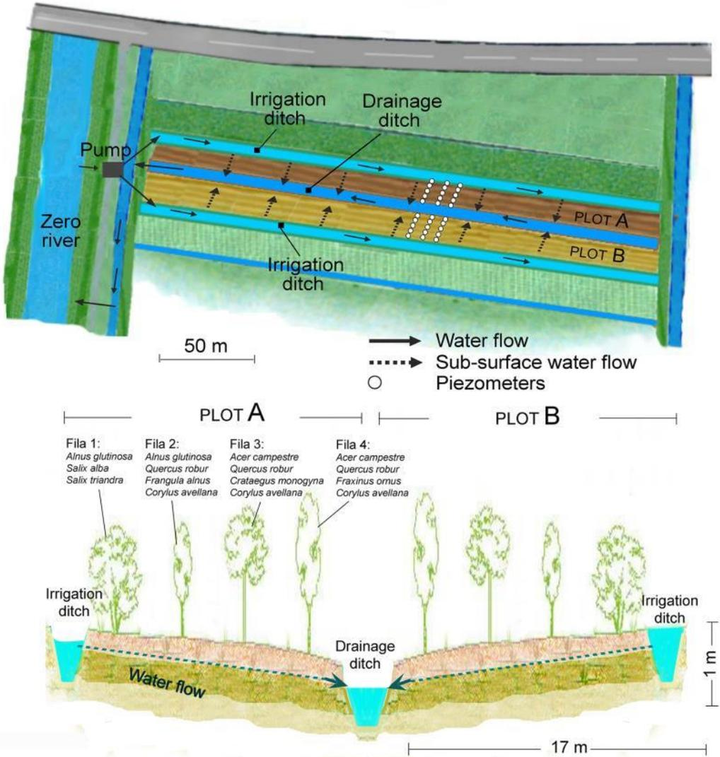
**Figure 14.** Plan (above) and section (below) of the 30 m wide experimental site: each plot is watered through an irrigation ditch carrying water from the Zero river. Soil setting allows a difference in elevation among the irrigation ditches (INPUT) and the drainage ditch (OUTPUT), resulting in a subsurface flow of water running through the wooded buffer strips (modified by Gumiero et al., 2011).
