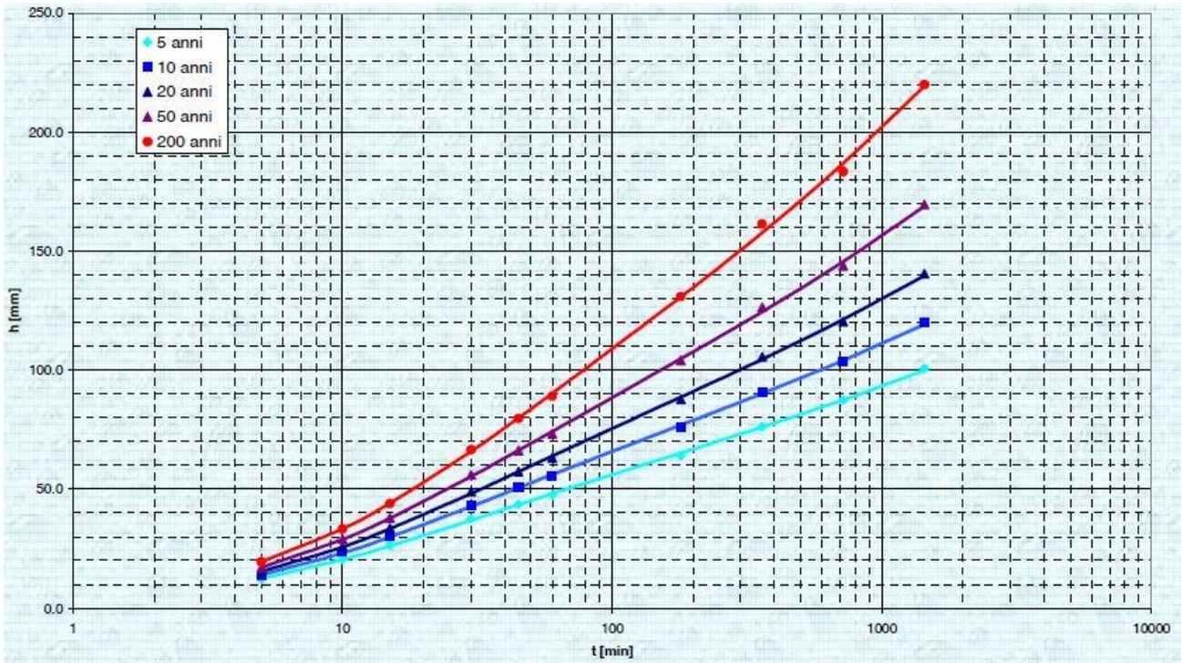
**Figure 39.** Rainfall depth-duration frequency curves function of different return times (5, 10, 20, 50, 200 years) for the homogeneous area South East coastal Area
