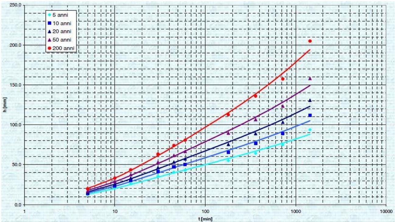
**Figure 40.** Rainfall depth-duration frequency curves function of different return times (5, 10, 20, 50, 200 years) for the homogeneous area North-East Area
