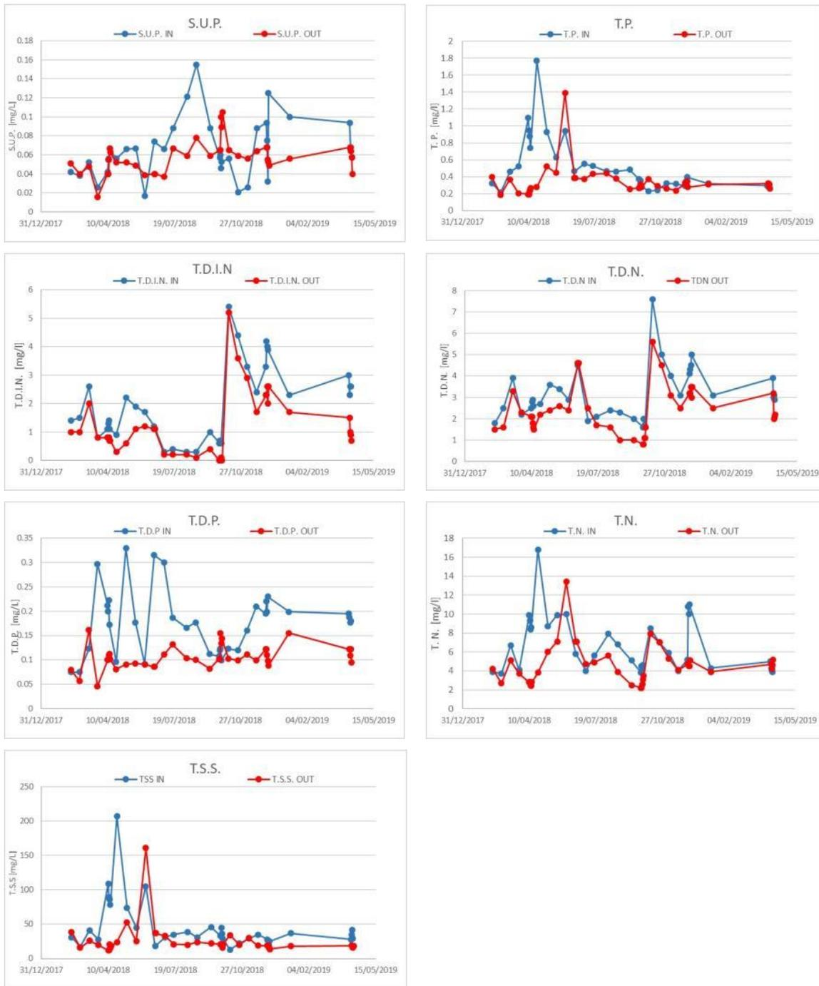
**Figure 41.** Influent and effluent pollutant concentration for the Rusteghin wetland
