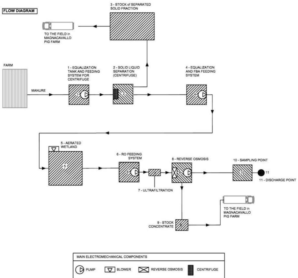
**Figure 5.** Flow diagram of the WWTP of Sasa Srl
