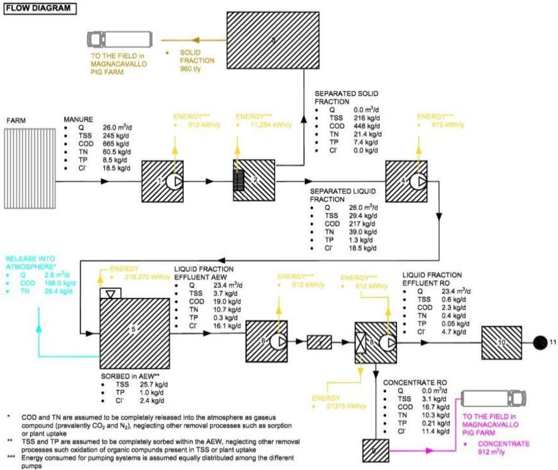
**Figure 8.** Mass flow diagram of the SASA WWTP
