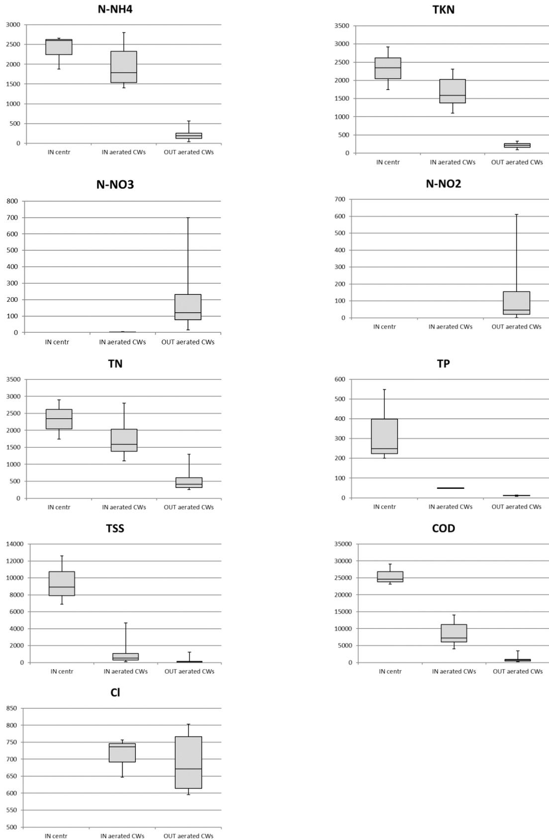
**Figure 10.** Box and whisker plots of the inlet and outlet concentration in the monitored pollutants: influent to the centrifuge, i.e., the primary treatment for solid-liquid separation; effluent from the centrifuge and influent to the aerated CW, i.e., the secondary treatment for the liquid fraction; effluent from the aerated CW.
