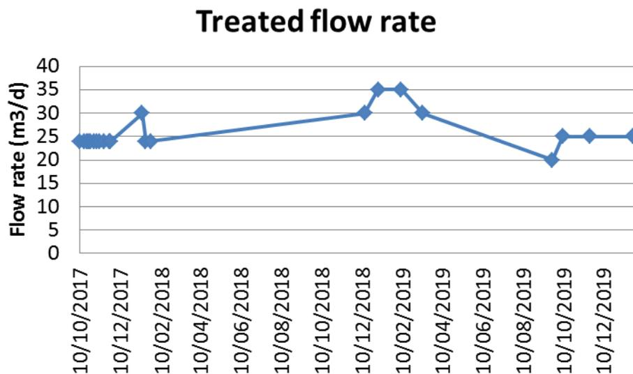
**Figure 11.** Treated flow rate at the SASA CW WWTP during the monitored period
