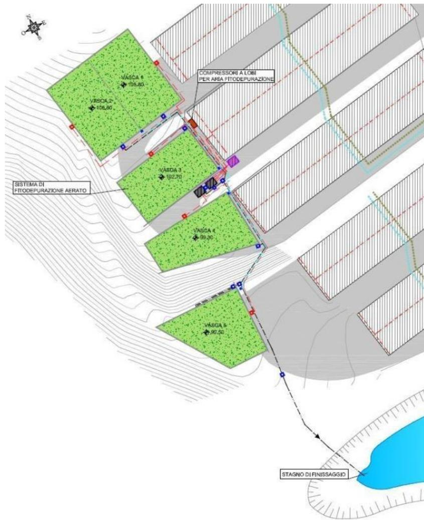
**Figure 4.** Planimetry of the aerated CW treatment plant of SASA Srl.
