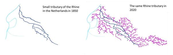
**Figure 28.** Changes in the drainage network occurred in a Dutch tributary of the Rhine between 1850 and 2020. Left: drainage network in 1850 (blue lines). Right: historical drainage (blue lines) and artificial drainage implemented since 1850 (pink lines)
