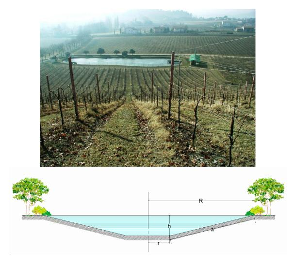
**Figure 25.** Above: example of a pond for the storage of water used for irrigation in the Lamone catchment. Below: example cross section of a pond designed with milder-sloped shores to enhance the provision of habitat.
