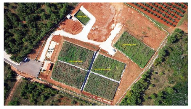
Figure 4. Aerial picture of the Kastelir WWTP, with indication of the treatment stages.
