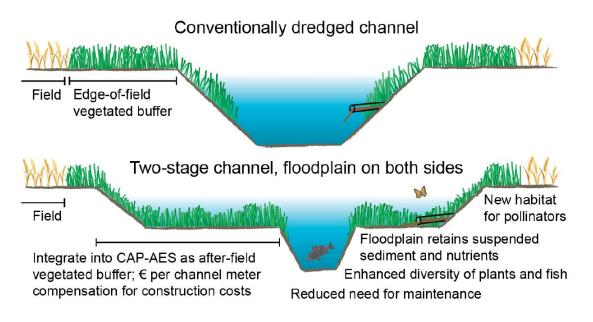
**Figure 22.** Characteristics of TSC design. From Västilä et al., 2021. CAP-AES means Agri-Envronmental Schemes under the Common Agricultural Policy of the EU.
