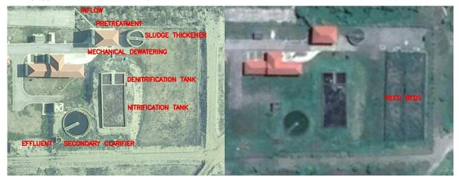
**Figure 5.** Aerial picture of Mojkovac WWTP before (left) and after RBs installation (right), from Google Maps<sup>™</sup>.
