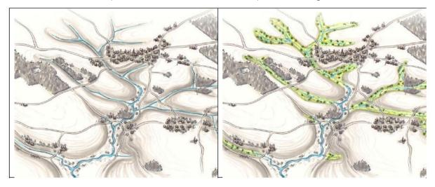
**Figure 29.** The concept of Natural Water Retention (sponge restoration) in upstream micro-catchment areas. Left: catchment in present conditions, with a high density of drainage. Right: reduction of drainage density through restoration of soil retention in small streams.
