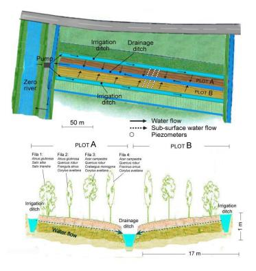
**Figure 12.** Plan (above) and section (below) of the 30 m wide experimental sub-site within the NICOLAS site: each plot is watered through an irrigation ditch carrying water from the Zero river. Soil setting allows a difference in elevation among the irrigation ditches (INPUT) and the drainage ditch (OUTPUT), resulting in a subsurface flow of water running through the wooded buffer strips (modified from Gumiero et al., 2011).
