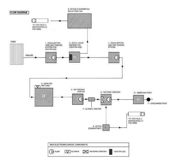
Figure 3. Flow diagram of manure management in the case study of San Rocco di Piegara.
