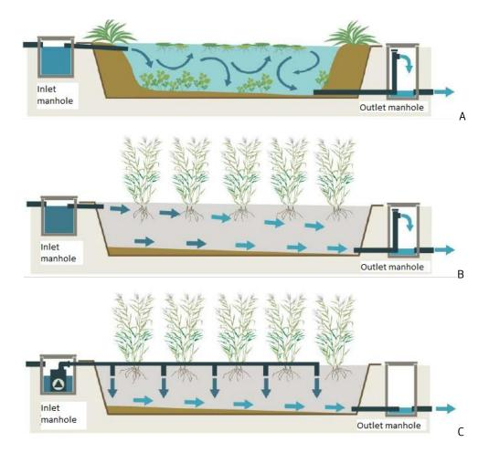
**Figure 1.** Cross-sections of constructed wetlands with free surface (A), subsurface horizontal (B), and vertical (C) flow. Source: original artwork by IRIDRA srl, in Pistocchi et al., 2020.
