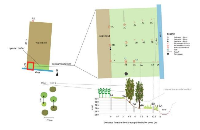
Figure 9. Illustrative design of the Scandolara buffer strip.
